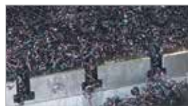
T-slots packed with difficult to remove chips
